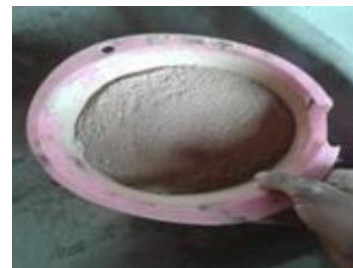
Fig. 6. Milled elephant grass being Sieved
